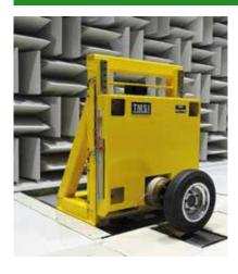
Anechoic Chambers are echo-free enclosures with a sound energy absorption level of 99% to 100%, or a reflected sound pressure level of 10% or less. The frequency at which the energy absorption drops below 99%, or the pressure reflection exceeds 10%, is known as the low-frequency cut-off. Sound absorption is obtained by lining the walls, ceilings, and floor with wedges or other sound absorbing elements or Super Soft panels, depending on performance level required and cut-off desired.
