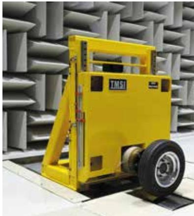
Anechoic Chambers are echo-free enclosures with a sound energy absorption level of 99% to 100%, or a reflected sound pressure level of 10% or less. The frequency at which the energy absorption drops below 99%, or the pressure reflection exceeds 10%, is known as the low-frequency cut-off. Sound absorption is obtained by lining the walls, ceilings, and floor with wedges or other sound absorbing elements or Super Soft panels, depending on performance level required and cut-off desired.
